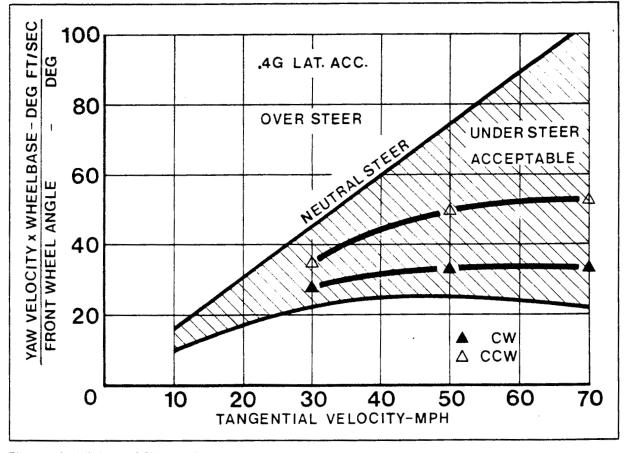
Figure 10. Minicars RSV steady-state yaw response.
