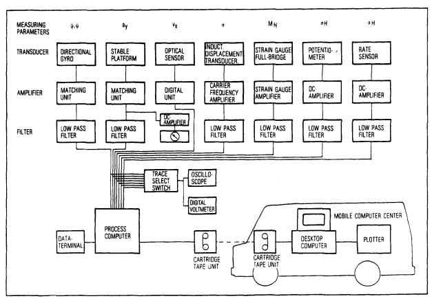
Figure 4. Minicars RSV measuring arrangement.
