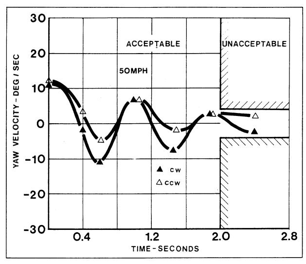
Figure 15. Minicars RSV returnability performance yaw rates at 50 mph.
