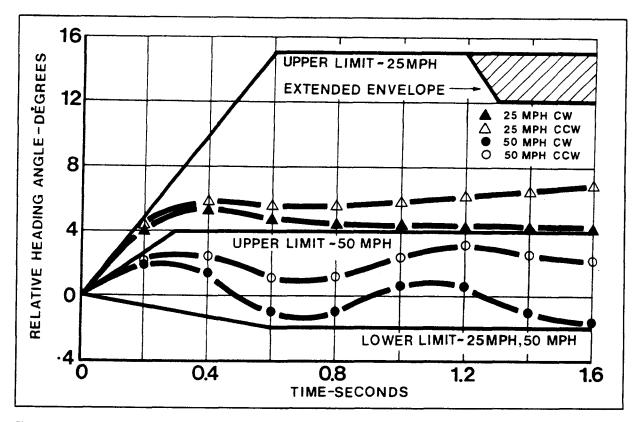
Figure 13. Minicars RSV Steering returnability free control heading.
