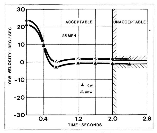
Figure 14. Minicars RSV returnability performance yaw rates at 25 mph.
