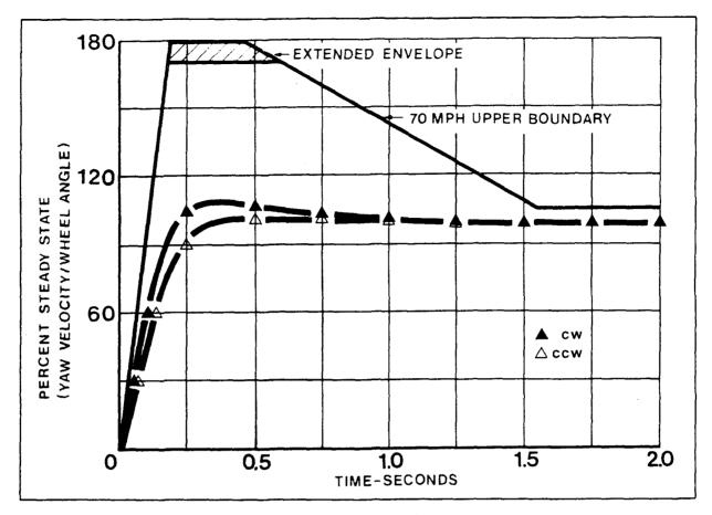
Figure 12. Minicars RSV transient yaw response at 70 mph.
