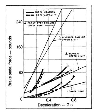
Figure 9. Minicars RSV brake pedal force versus vehicle deceleration.
